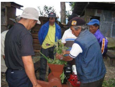
Improvement of composting with locally manufactured grass shredder (2008)
